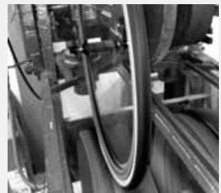
Tire Durability Test 80kg @ 40 kph
